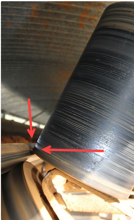
Fig.18: 5-Support with 5 rollers: the belt heel comes up against on roller edge
