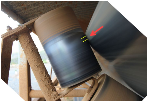
Fig.16.1: Carcass too rigid for a deep trough.
